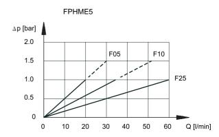
NOTE 2: The filter size has to be selected so that with the nominal flow rate the pressure drop is lower than 0.8 bar.
